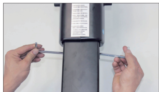
Tighten the screw with two #A wrenches turn simultaneously.
