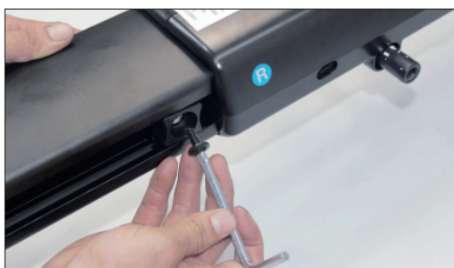
Tighten #14 screw to rail with the phillips end of #A wrench.
