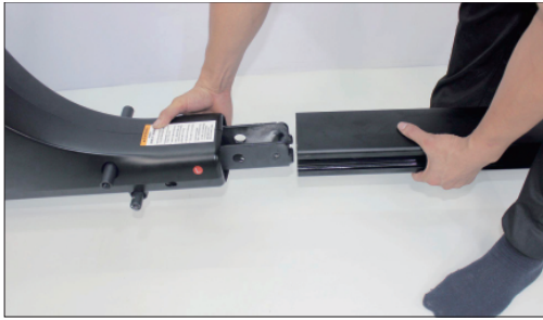
Connect the rail with main frame as photo shows.
