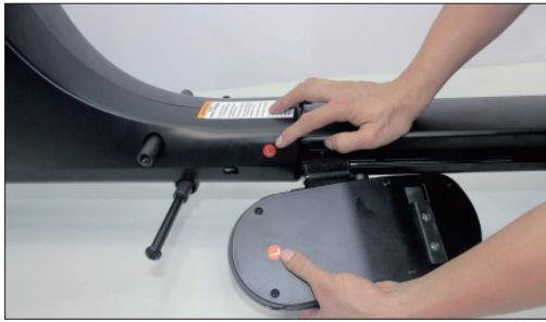
Prepare left pedal and check if the L label is the same as the one on main frame.
