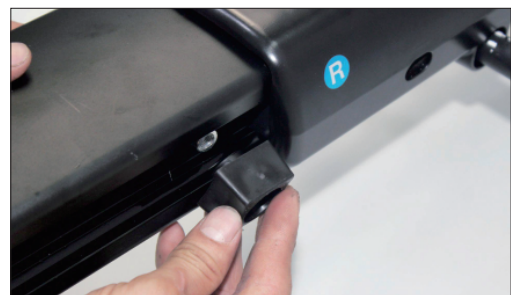
Assemble another #13 rubber pad to another side. (The arc should be on left & right side).
